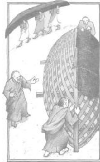
3. The monks prepare their boat. A wooden frame is covered with skins just like the currachs of today. However, the monks added sails and covered over the top, making the boat seaworthy on very long journeys.
